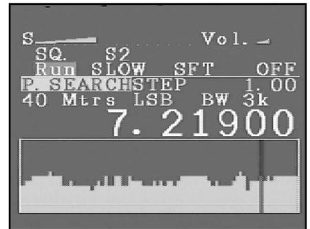
Figure 8—The AR7000B band scope in the search mode. The band limits, search name (40 Mtrs in this example), mode, step size, bandwidth, sweep direction and pause duration can all be varied in a setup menu.
