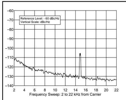
Figure 4—Worst-case HF spectral display of the IC-706MKIIG transmitter output during composite-noise testing. Power output is 100 W at 14.02 MHz. The carrier, off the left edge of the plot, is not shown. This plot shows composite transmitted noise 2 to 22 kHz from the carrier.
