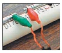
Figure 4—Close-up showing the connection that allows the Q&D antenna to be used as a center-fed dipole.
