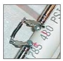
Figure 3—The shorting bar that enables the antenna to be used as a 12 foot vertical.
