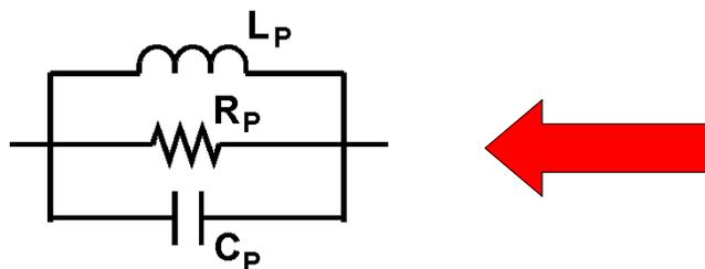
Data Sheets Use This Equivalent Circuit to Graph the Impedance
