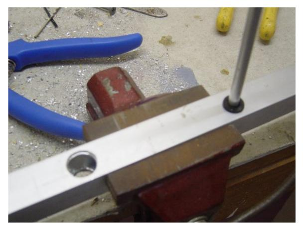
The boom was drilled using a drill press for accurate ling ups, elements cut to size, and LED inserts trimmed. It was time to put it all together.
