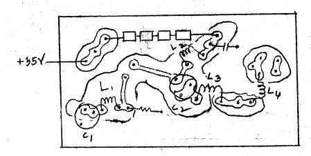
For those of us who are using the home - brew 2-M transreceiver which has an output of 1 watt (approx.), the power output can now be increased three fold in a simple Low Cost way.
