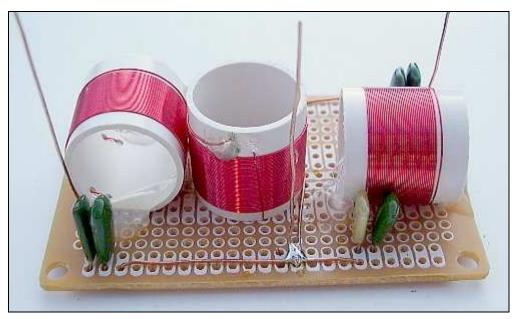
This filter works with 50 ohms in/out, for which the loop antenna is more or less matched. If you use it with some other antenna, a tuner may be necessary.
