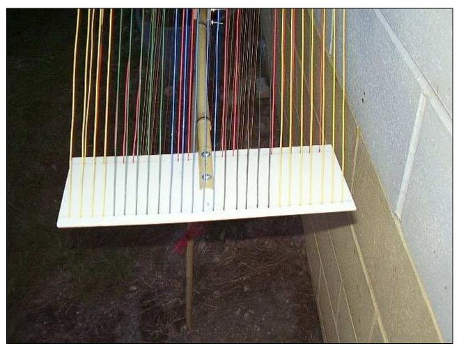
The loop wire is insulated, stranded stuff scavenged from long runs of security camera cables. THAT was a pain to strip and recover! I read that the ideal wire length for this kind of loop is 0.085 wavelength - which the total amount of wire turns out to be at 255KHz, pretty much band-centre of interest.
