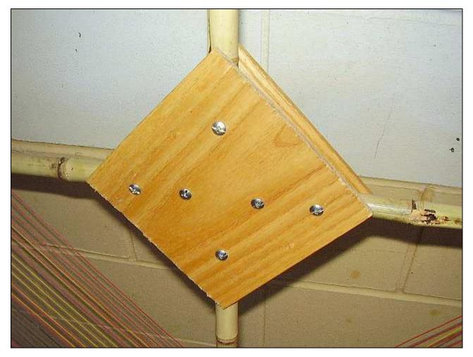
The hub plates are made from 3/16" ash thins for scroll sawing that I oiled for weather resistance. The arms and mast are formed from bamboo poles from a garden store. Strong and light!
