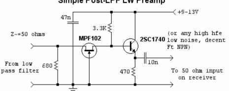
Circuit noise appears to be well below the noise level of the LW band, so that switching it in/out makes zero audible difference in the noise floor. No tuned circuits or coils... this is LF after all.
