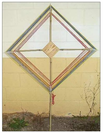
I just finished a small (69cm per side) quad loop for use from 150 - 430KHz that came amazingly close to the math prediction. I wound it for Non-Directional Beacon DXing...taking full advantage of the minimal sunspots recently, which makes for great LW DX.
