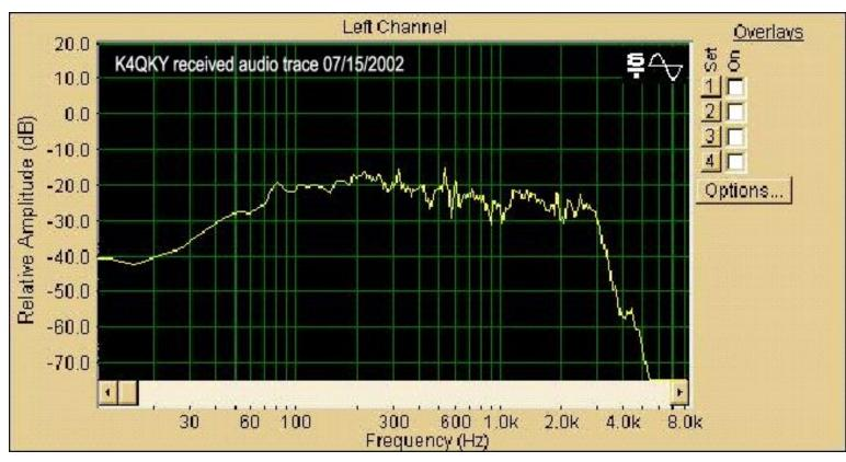
Balanced (flat) frequency response from 70 hz to 3.0 khz
