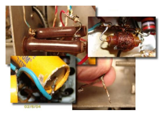
Numerous physical defects were found and repaired/replaced during this step including (clockwise from top left) poor solder connections on two parallel wire round resistors, overheated choke, questionable electrolytic capacitor and several broken solder wire connections. A broken microphone connector (not shown here) was also replaced. The VFO tuning linkage was completely disassembled, cleaned and lubricated. All switches and contact points were cleaned with "De-oxit".
