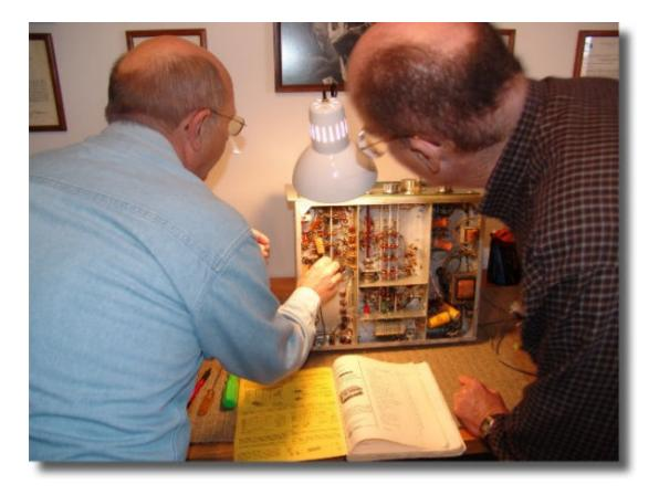
K4ENE "Don" and KJ4W "Bill" inspect the components beneath transmitter's chassis. All tubes (lower center photo in the montage) were tested with seven (including both 6146 power amp tubes) requiring replacement.
