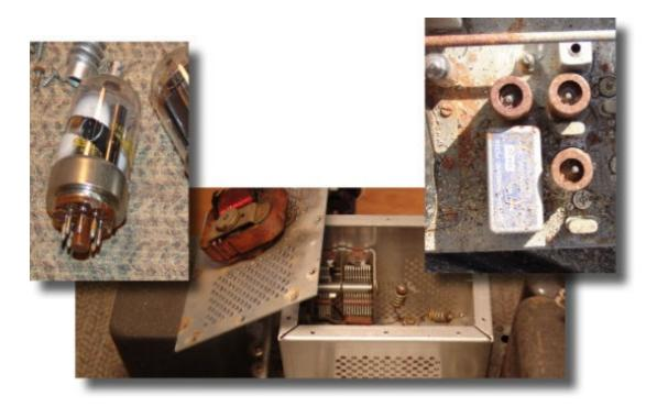
Chassis corrosion and debris accumulation over the years. Note the cracked 6146B power amplifier tube in the left of this photo montage.
