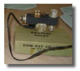
Note: Dow Key Relay model DK60G2C 52 ohm 1000 Watts 115v to switch transmit and receive between the Valiant transmitter and Hammarland SP-600 receiver. This particular model has a separate set of contacts to mute the receiver. Click <u>here</u> for specifications.
