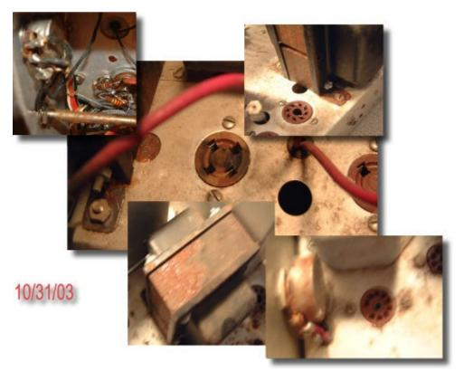
Chassis corrosion most likely resulting form moisture accumulation over the years. Note the evidence of arching of the one of the 866 Mercury Vapor H.V. Rectifier tube sockets in the center of this photo montage.
