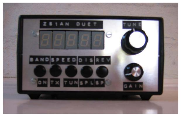
**Figure 7 - Front Panel Layout**
