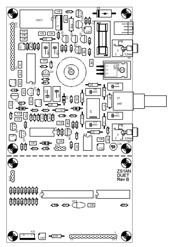
Figure 4 – Parts Placement Diagram (Top of Board)
