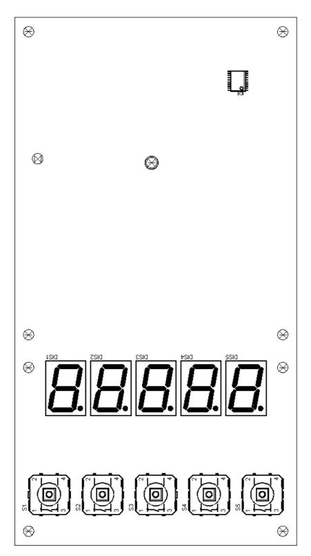
Figure 5 – Parts Placement Diagram (Bottom of Board)
