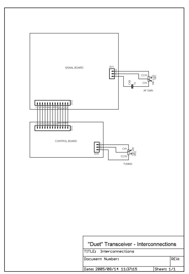
Figure 6 – Interconnections between the control board and signal board
